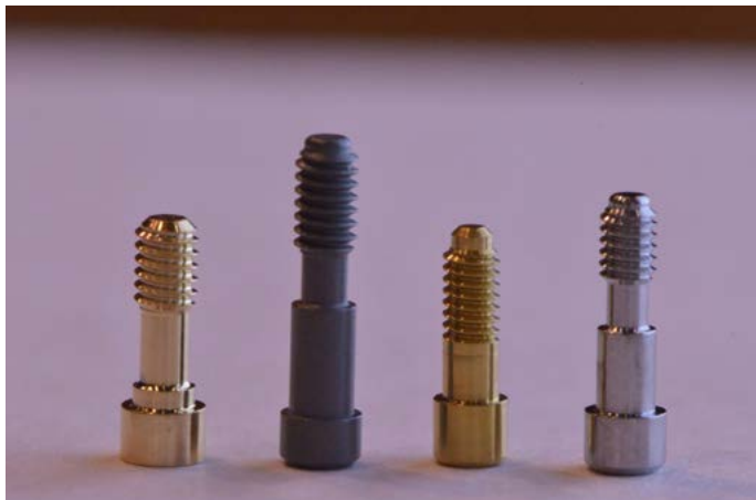
Fig. 1 Screws with different surfaces require different tightening protocols. From left to right: Anodized, DLC (diamond like coating), 23 Carat Gold, Titanium Alloy
