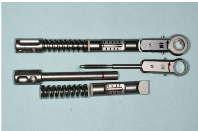
Fig. 2 Manual toggle wrench. Post use it must be disassembled, oiled, then re-assembled and stored in a zero torque state.
